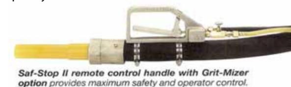
*Saf-Stop II remote control handle with Grit-Mizer option provides maximum safety and operator control.*
